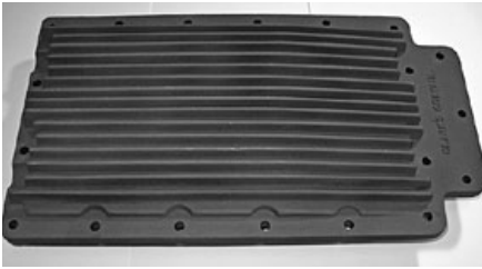
The newest Clark's pan is finned on the bottom side to maximize temperature shedding.
