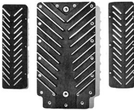
Otto Parts finned oil pan and rocker covers are black anodized to improve cooling efficiency. Pan has 314 square inches of cooling surface area; covers add another 316 square inches.
