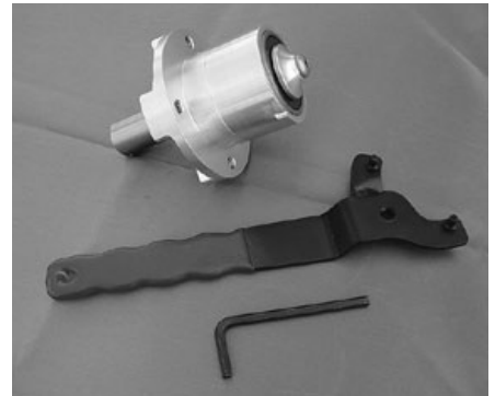
As assembled. The special tool holds the fan bearing in place as you remove the top retainer.
