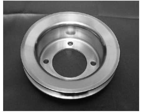
This aluminum fan drive pulley from American PI replaces the stock, stamped-steel unit.
