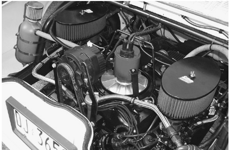
Brian O'Neill's track car uses an electric motor drive for a full-size fan. Proven in cool weather, it has yet to be tested in hot conditions.
