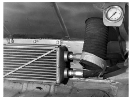
Doug Roe's Spyder-engined "Desert Rat" never exceeded 260° F oil temperature in a one-hour race in 90° ambient temperature using Harrison "big car" oil cooler installed as you see it here. Body is cut away behind cooler for airflow. Hose is cool-air inlet for carburetor.
